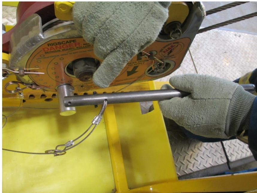
2.1.6. Check to see that the spring pin is properly inserted into the override-brake handle.
