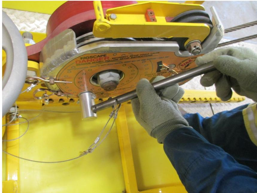
2.1.7. Insert handle into the override-brake hub.
