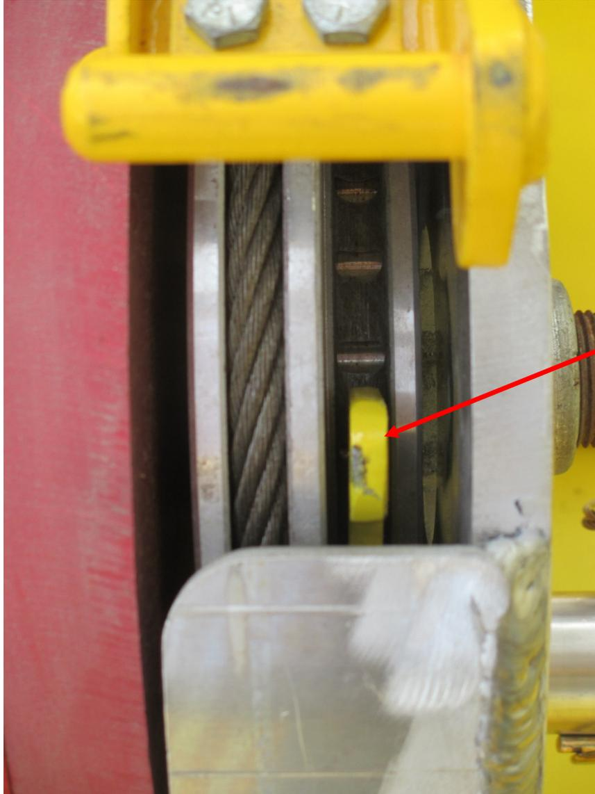
2.1.11. The override brake pad (arrow) should ride the center of the outer sheave.
